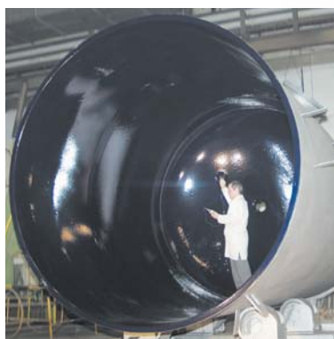
Split vessel, diameter 3000 mm, capacity 26000 litres (Wacker-Chemie)
