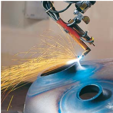
Computer-controlled flame-cutting robots guarantee high-precision synchronous cutting resulting in precise fitting accuracy of neck and nozzles
