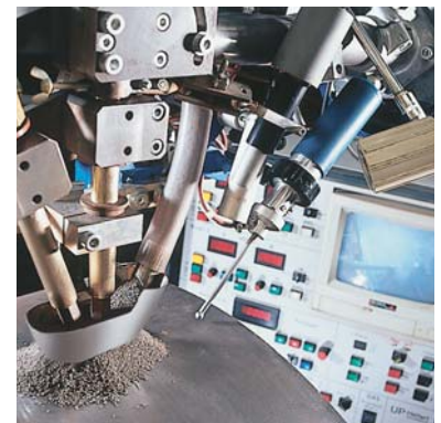
Our submerged-arc automatic welding machine does material-friendly welding based on minimal heat effect for up to 100 m of weld seams per unit
