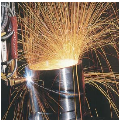
Computer-controlled flame-cutting robots guarantee high-precision synchronous cutting resulting in neck and nozzles that fit with absolute precision
